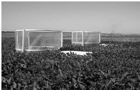
Fig. 6 - The cylindrical form of an OTC [from CRA – SCA (Agricultural Research Council – Research Unit for Cropping Systems in Dry Environments), 2006].
