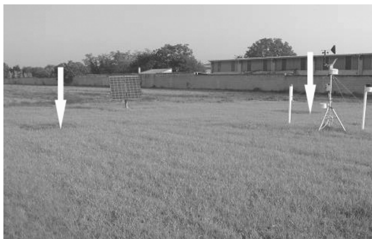
Fig. 9 - The meteo-lysimeter experimental site, arrows indicate the mini-lysimeters
