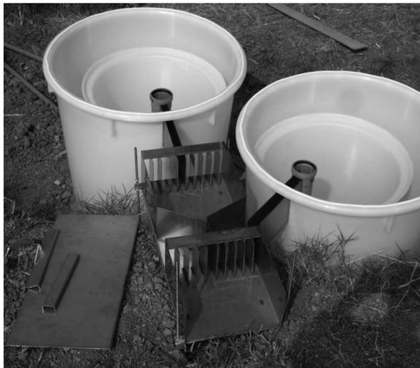
**Fig. 1** - Multislot divisor with tanks.
