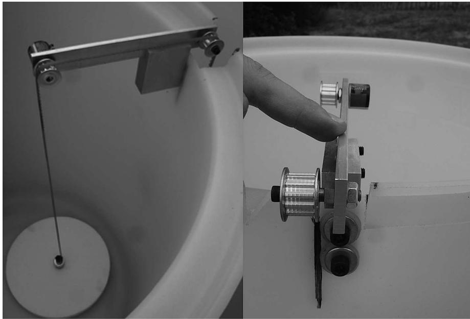
**Fig. 2** - Floating level system.
