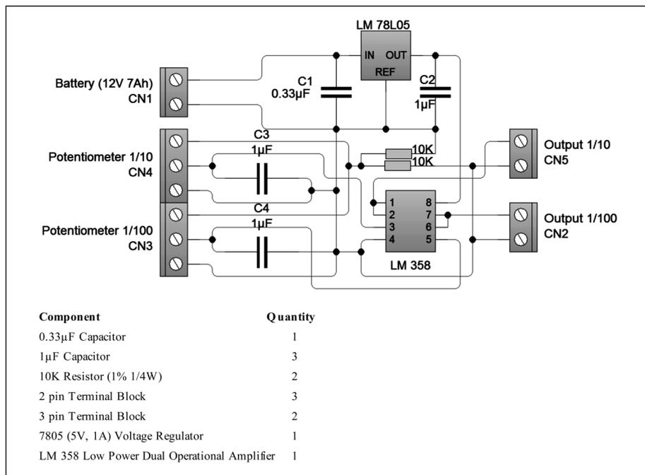
**Fig. 3** - Scheme of the signal condition system and component list.
