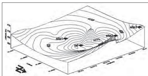
Fig. 1 - The Volturino catchment with the 4 measurement points. Reference site in plane at the bottom of the catchment; Site1 NW exposed, orientation of the plot (O) 310°, slope of 9°, 7 m is the difference in altitude from the reference; Site2 SE exposed, O 125°, slope of 6°, 12 m; Site3 SE exposed, O 120°, slope of 1°, 18 m.
