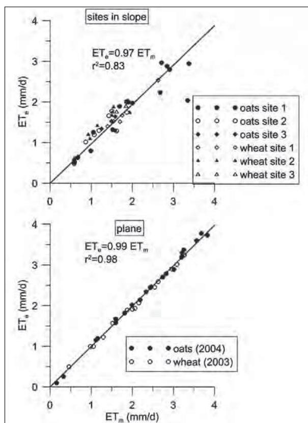
Fig. 2 - Comparison, for wheat and oat, between estimated and measured  $ET$  at daily scale, for all sloped sites, and the reference site in plane.
