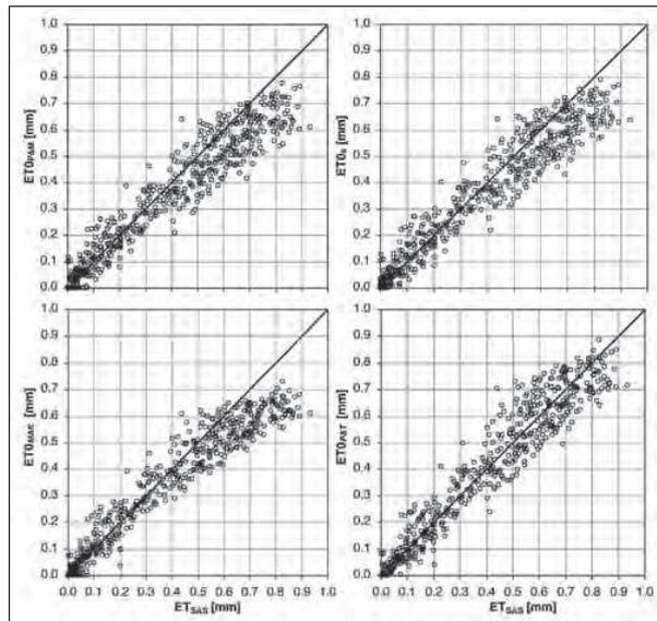
Fig. 1 - Comparisons of hourly measured,  $ET_{SAS}$ , with estimated using Priestley-Taylor ( $ET_{P\&T}$ ), Makkink ( $ET_{MAK}$ ), FAO modified 24-h Penman-Monteith equation ( $ET_{P\&M}$ ) and ASCE-EWRI's standardized Penman Monteith ( $ET_0$ ) models.
