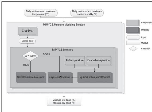
Fig. 1 - MIMYCS.Moisture modelling solution component diagram.
